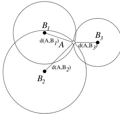
**Fig. 3.** A sensor at  $A$  not equipped with a GPS device can determine its position from the positions of its three neighbors  $B_1, B_2, B_3$ .
