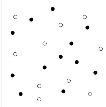
**Fig. 7.** Sensors dropped randomly and independently over a unit square region. Bolds (respectively, empty) circles denote sensors which are equipped (respectively, not equipped) with GPS devices.
