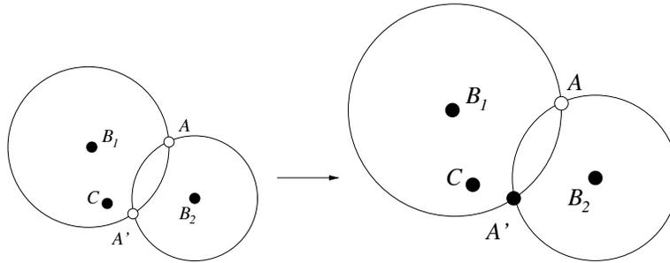
**Fig. 4.** Application of 3-NA will equip node  $A'$  with its  $(x, y)$ -coordinates, but it fails to do it with node  $A$ .
