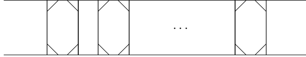
Fig. 3. A guillotine subdivision with n = 6k + 2 segments that requires 4k \theta -transmitters. Each of the 4k triangular faces must have a \theta -transmitter on its boundary and no two triangular faces share a boundary.
