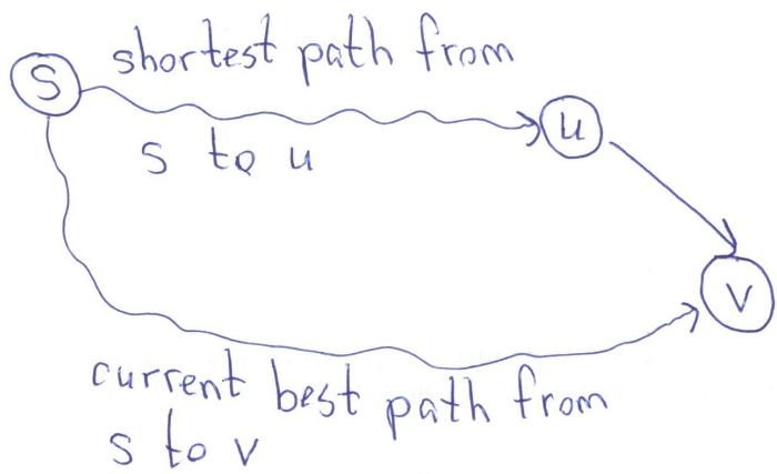
$$d(v) = \min(d(v), d(u) + \text{wt}(u,v)).$$
