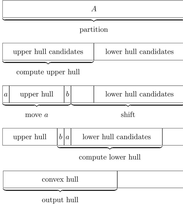
Fig. 2. A faster implementation of GRAHAM-INPLACE-HULL.
