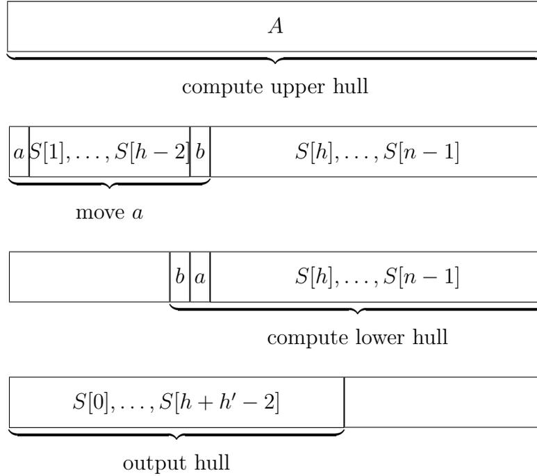
Fig. 1. The execution of the GRAHAM-INPLACE-HULL algorithm.
