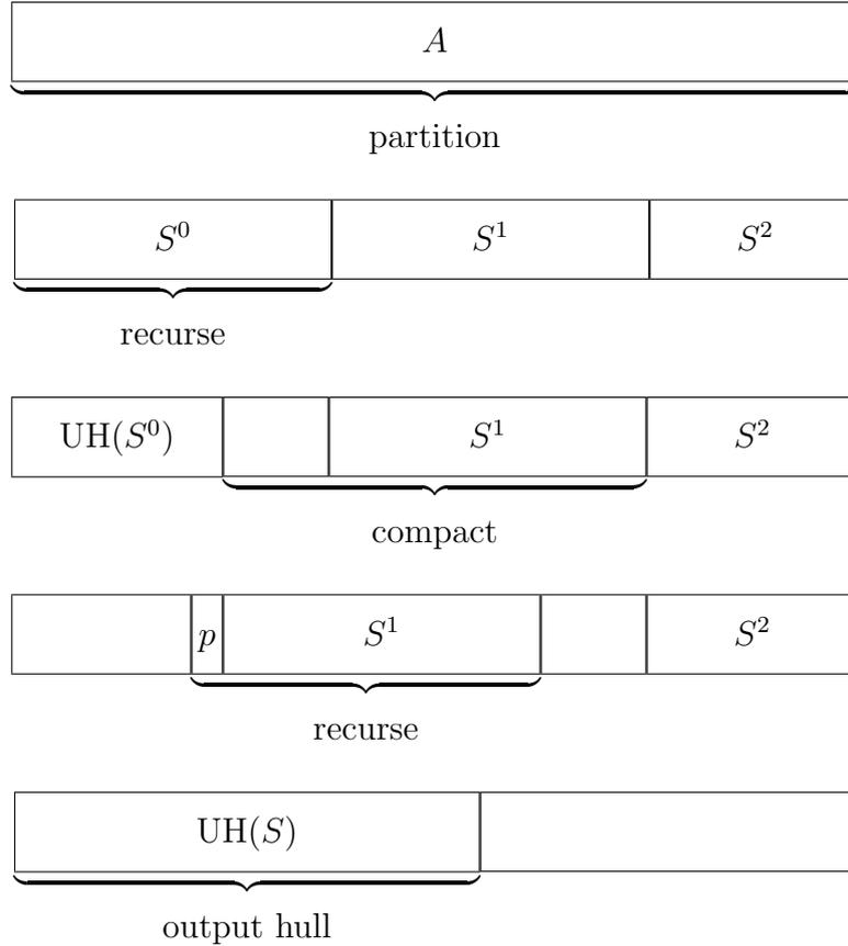
Fig. 5. Overview of the CSY-IN-SITU-HULL algorithm.
